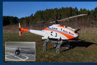
Landing on moutainous or pitching surfaces could be much safer with Rotor Buzz's flexible "legs" landing gear.
